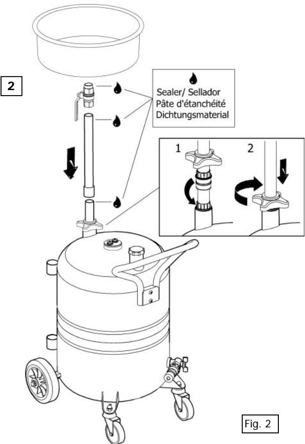
(GB) Assemble the tube with the funnel and fix the assembly on the tank.
